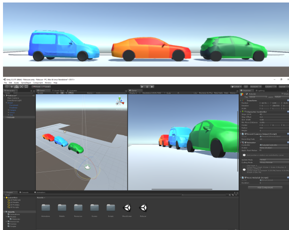
Figure 2: 3D simulation framework. At top, a side view of the 3 cars. At bottom, the scene setup in Unity3D including the visualization and images generation parts. The simulator handles pedestrian simulated trajectories and point of views. Usage of a flat color shader to generate the images allows to easily segment and identify the visible parts of each car.
