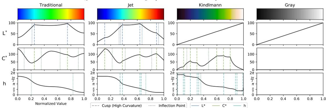
**Figure 3:** The CIELCh lightness ( $L^*$ ), chroma ( $C^*$ ), and hue ( $h$ ) profiles for the four color maps we looked at in our exploratory study, with dotted and dashed lines showing the derived locations of cusps and inflection points.
