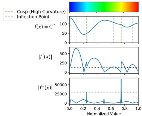
**Figure 5:** Deriving the chroma ( $C^*$ ) indicators for the traditional rainbow color map: (upper) the cubic spline approximation of the chroma profile, (center) the derived gradient magnitude, and (bottom) the derived curvature magnitude. Horizontal lines show the thresholds used to isolate the cusps and inflection points, which are represented by the vertical lines overlaid on the chroma profile.
