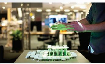
▶ Recompose: Direct manipulation and gestural interaction with 2.5-D shape display.
