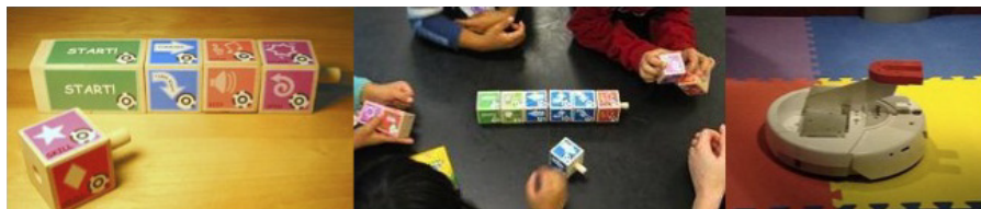
Fig. 4.8 Tern [103] is a tangible computer language designed for children in educational settings. Tern is featured in a permanent exhibit at the Boston Museum of Science called Robot Park. From left to right: Tern’s blocks, collaborative programming using Tern, the programmable robot at the Robot Park exhibition (Photos: courtesy of Michael Horn).
