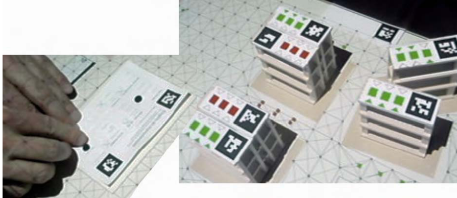
Fig. 4.6 Tinkersheets [267] supports learning about warehouse logistics and enables users to set simulation parameters through interaction with paper forms where small black magnets are placed onto parameter slots (photo: E. Hornecker).
