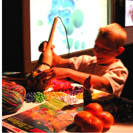
Fig. 4.11 I/O Brush [205] is a physical drawing tool to explore colors, textures, and movements found in everyday materials by allowing users to “pick up” images and draw with them (photo courtesy of Kimiko Ryokai).
