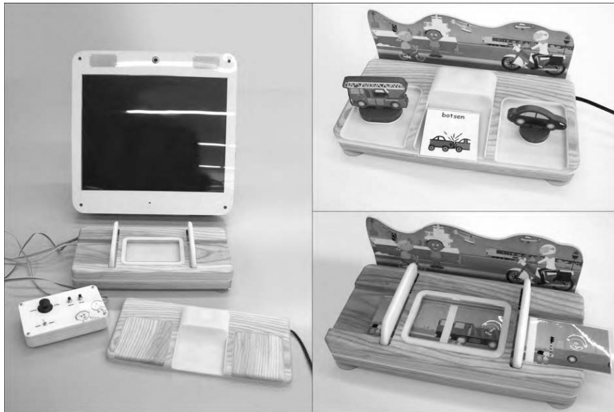
Fig. 4.3 Linguabytes [94], a TUI for improving speech-therapy sessions with severely impaired children. Left: the overall system, including the control unit for the therapist and a monitor that displays animated sequences in response to the child's actions. Right, Bottom: a storybook is sled into the top rim of the board, activating a subunit, here on traffic. The booklet can be moved back and forth. Placed behind the unit, a corresponding scene is triggered as an animation with audio on a screen. Top: The trays recognize the wooden images placed onto them. In this unit the objects are combined into sentences to train syntax (photo: Bart Hengeveld).
