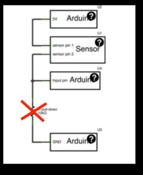
if direct connection, short circuit between 5V and GND when sensor activated
