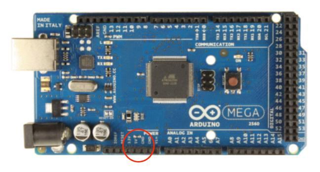
Analog (=continuous) input pins
