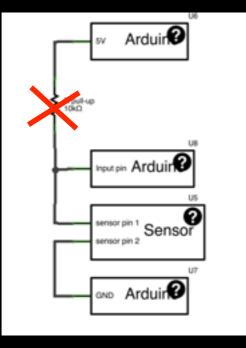
if direct connection, short circuit between 5V and GND when sensor activated
