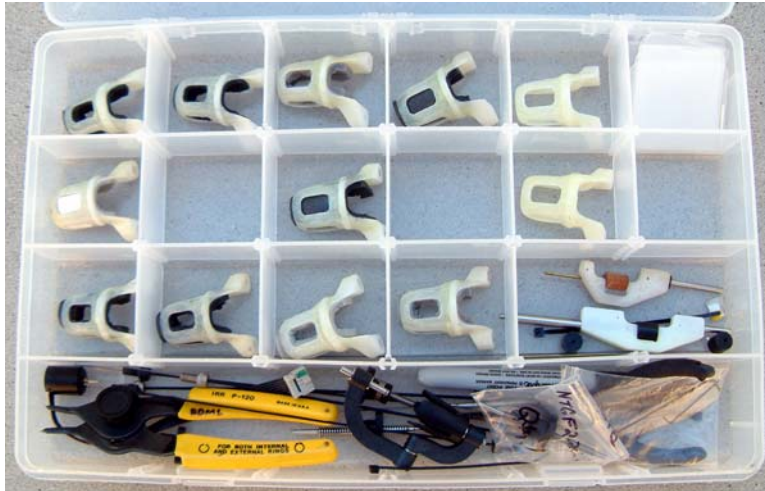
Figure B-7. A family of thimbles were used to accommodate the wide range of finger sizes. The thimbles are lined with 1/6 inch, 1/8 inch, or 3/16 inch PVC foam tape. The thimbles also differ based on the vertical offset from the bottom of the user's finger to the centerline of the push-pull wires.
