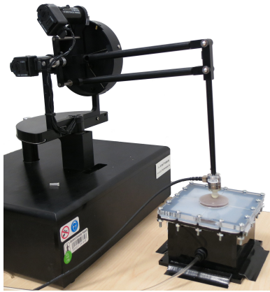
Figure 3: Setup used to measure force-deflection data for a single haptic jamming cell. A force/torque sensor was attached to the end effector of a Phantom Premium robot and was used to manually palpate the center of the cell. Position data was recorded from the Phantom Premium.
