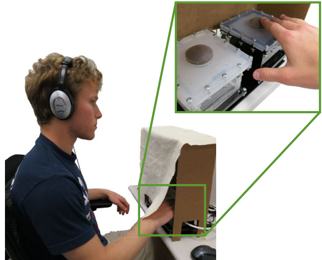
Figure 4: A subject interacts with the experimental apparatus. Two single-cell devices were placed side by side and covered by a curtain. Subjects were asked to state which device presented a larger stimulus (either rigidity or size) based on touch alone.
