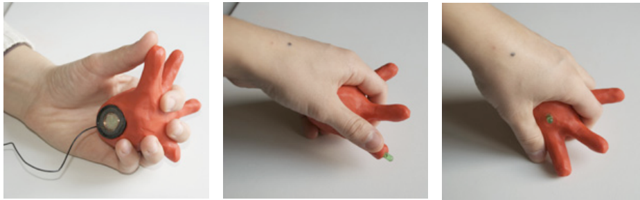
Fig. 10. Design alternatives for output ports: sound (left), light (LEDs in center and right). Focusing on the output ports: according to the way the tool is handled by the user, the lights may be hidden or not.
