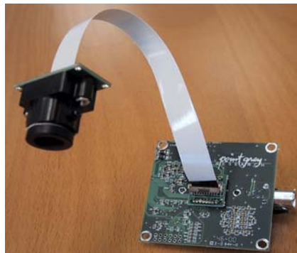
Figure 2: Assembled extended head camera
