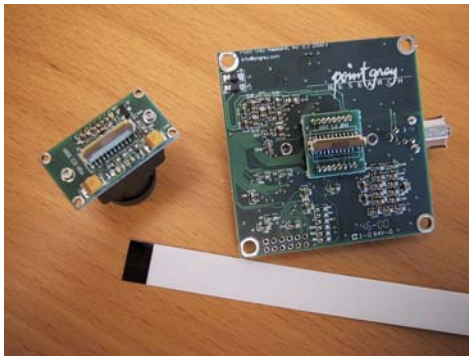
Figure 1: Unassembled extended head camera
