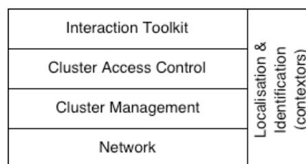
Figure 4: **I-AM software architecture layers decomposition**
