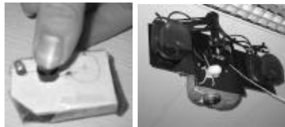
Figure 4: On the left, the “GLOSS clicker”, a wireless “home made” pointing instrument that includes a press button and a LED mounted on top of a 2X4 cm foam box wrapped with paper. A battery embedded in the box provides power to the LED. On the right, a GLOSS system actuator (video-beamer) and two camera sensors.
