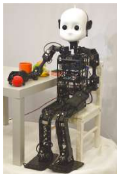
NICO – Neuro-Inspired COmpanion: A Developmental Humanoid Robot Platform for Multimodal Interaction http://nico.knowledge-technology.info
