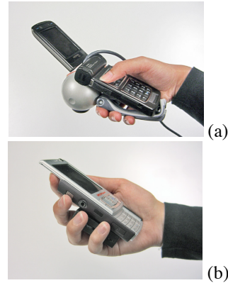
Fig. 8. (a) The webcam with Nokia N93 for moving the 3D character. (b) The SHAKE with Nokia N95 for 3D object examination.
