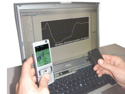
Fig. 3. OIDE Debugging and Logging tools. In the example, the Shake accelerometer events are logged in order to tune the interaction with the mobile game.
