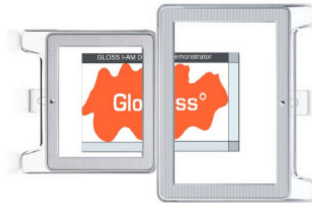
Figure 4. Top-to-Top composition: two surfaces are coupled via their top edges.
