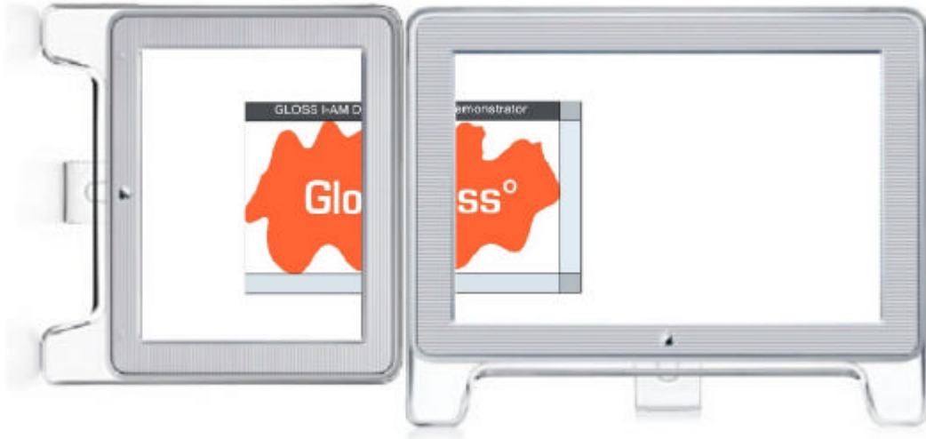
Figure 8. Top-to-Left composition: The top edge of one surface is coupled to the left side of the other.
