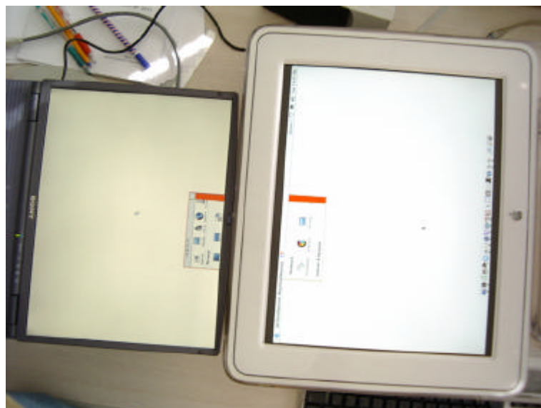
Figure 2. A window displayed on a multi-surface interaction space composed from a PC screen and of an Apple screen connected via their top edges.
