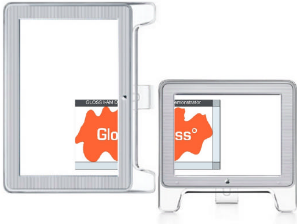
Figure 6. Bottom-to-Left composition: The bottom edge of one surface is coupled to the left side of the other.
