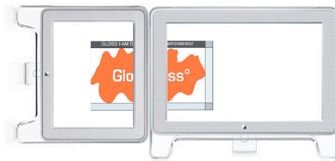
Figure 4.12. Top-to-Left composition: The top edge of one screen is coupled to the left side of the other.
