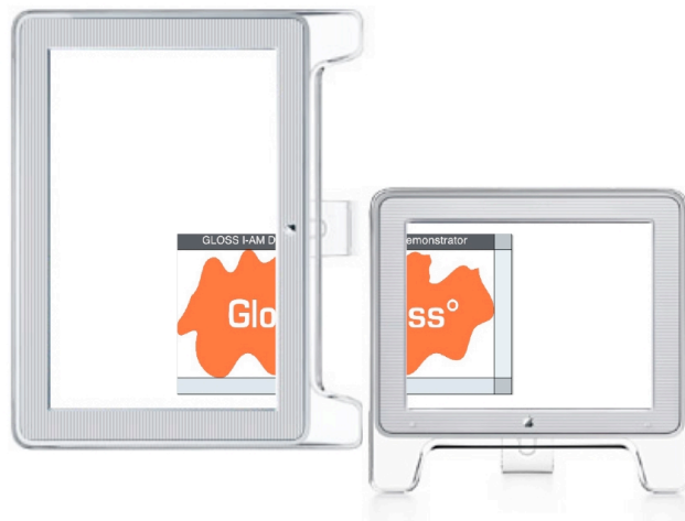
Figure 4.11. Bottom-to-Left composition: The bottom edge of one screen is coupled to the left side of the other.
