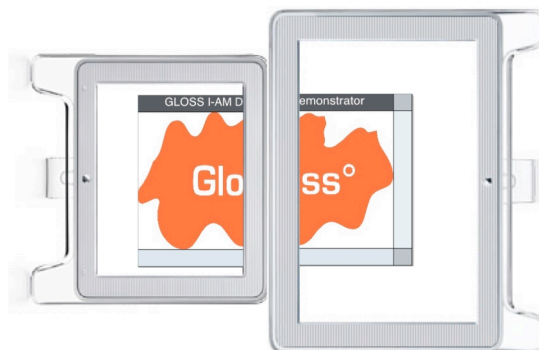
Figure 4.10. Top-to-Top composition: two screens are coupled via their top edges.
