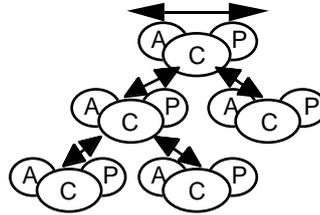
Fig. 3. In the PAC style, PAC components are configured hierarchically using event-based connectors. Arrows illustrate the information flow (vertical flow between agents, horizontal flow between the facets of an agent).
