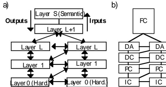
Fig. 1. a) Dewan's generic architecture for multi-user systems. Arrows denote information flow. b) An instantiation of Dewan's model using the functional layers of Arch. Here, the functional Core FC is shared while each branch is composed of a Domain Adapter DA, a Dialogue control Component DC, a logical Presentation Component PC, and a physical Interaction Component IC.
