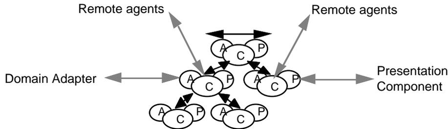
Fig. 4. A Dialogue Component in PAC\* and its connectors. Dark arrows denote connectors within the Dialogue Component. Dimmed arrows represent connectors with other components.
