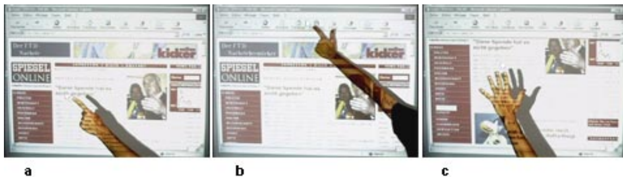
Figure 6.1: The FingerMouse on a projected screen (a) Moving the mouse pointer (b) Double-clicking with an outstretched thumb (c) Scrolling up and down with all five fingers outstretched
