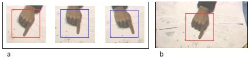
Figure 3.4: Correlation tracking with rotation (a) Original (middle) and rotated sample patterns. (b) The found object most resembles the left-rotated pattern.
