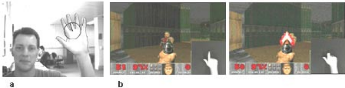
Figure 2.4: Contour-based hand tracking (a) Hand contour extraction (from [Heap 95]) (b) Sequences from a Doom game controlled by hand (from [Segen 98])
