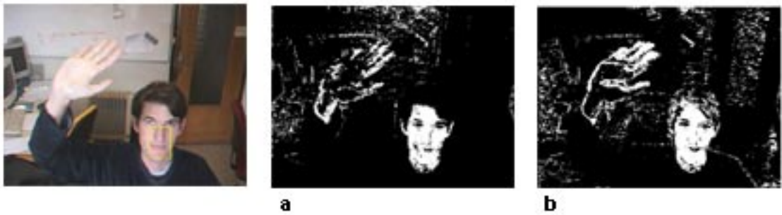
Figure 3.2: Generalized color models (a) Color space transformation (b) Gaussian function
