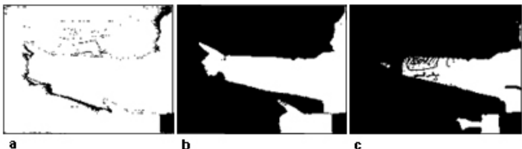
Figure 3.6: Thresholded difference images (a) Insufficient threshold of 5% shows background noise (b) “Right” threshold of 25% (c) Threshold of 75% cuts off the hand
