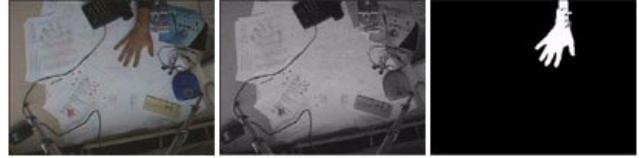
Figure 2. Image differencing with reference image. From left to right: input image, reference image, output image.
