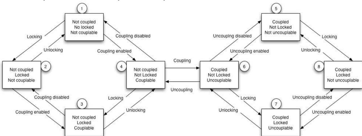
Figure 7. Coupling  $(e1, c, e2)$  as a Finite State Automaton. For the sake of readability, the transitions between states 1 and 3, 2 and 4, 5 and 7, 6 and 8 are not represented.
