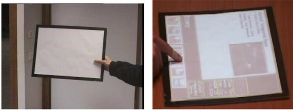
Figure 6. A piece of white cardboard with black borders as a potential interactive surface (left). The cardboard transformed into an interactive surface when coupled with the SCP (right).
