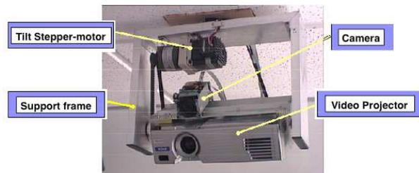
Figure 5. The Steerable Camera-Projector (SCP) pair.
