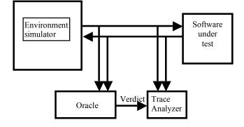
Lutess automatically builds a test data generator and a test harness which links the generator, the software under test and the oracle, coordinates their execution and records the sequences of input-output values and the associated oracle verdicts.
