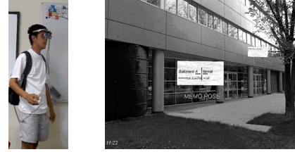
Figure 1 : Left: A Memo user, equipped with the HMD and holding a mouse. Right: A View through the HMD: The user is in front of a building and can see two digital notes
