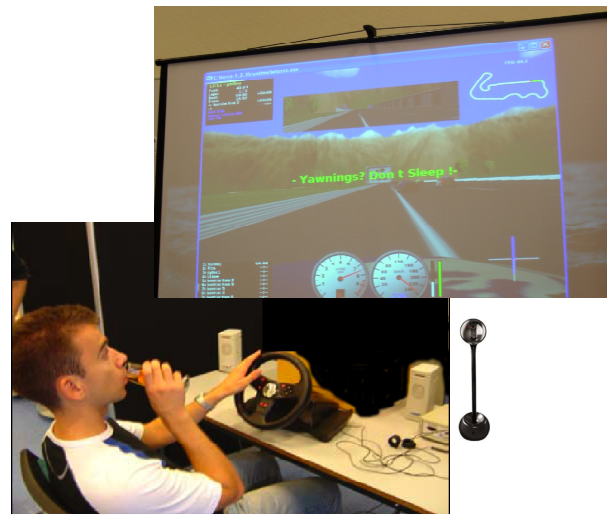
Fig. 3. Multimodal driving simulator: demonstrator in use.
