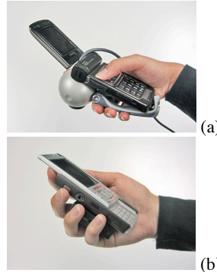
Fig. 8: (a) The webcam with Nokia N93 for moving the 3D character. (b) The SHAKE with Nokia N95 for 3D object examination.
