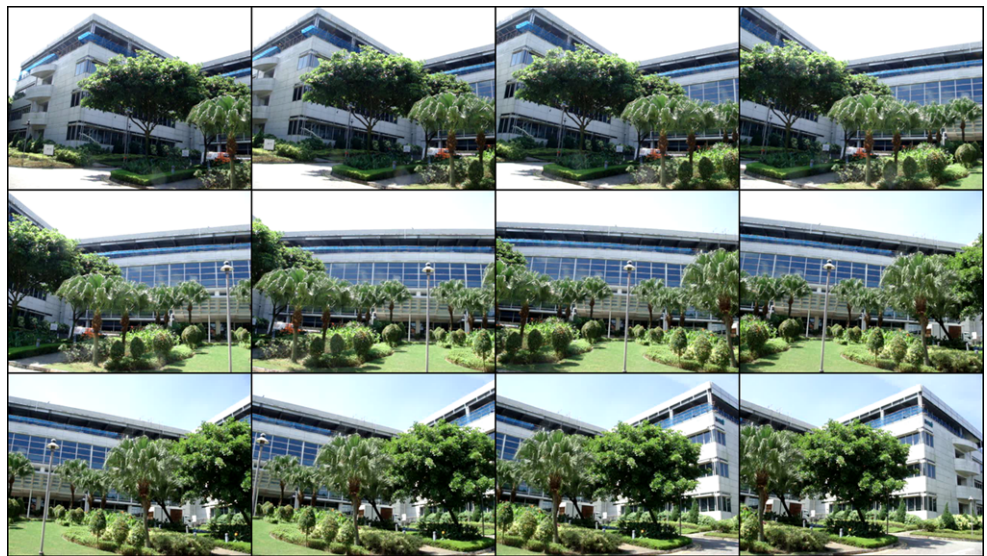
Fig. 5 Capturing the facades of a large structure by recording a video. The video frames contain a lot more information about the structure than a few images
