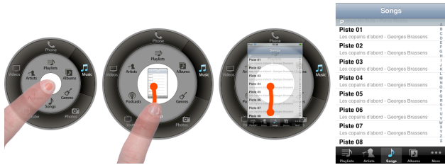
Figure 3: Long lists management: the linear list appears in the center of the Wavelet menu and is surrounded by its parent menus.
