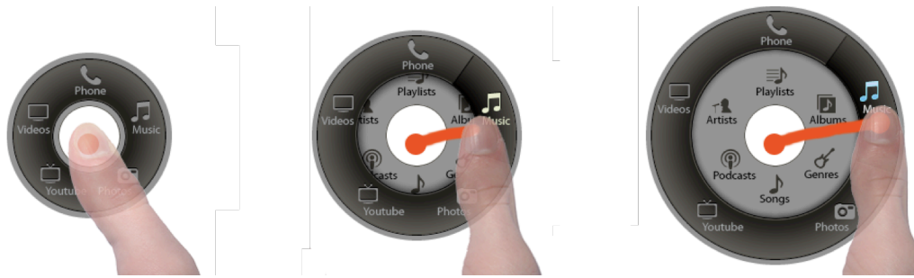
Figure 2: The Wavelet menu appears centered around the contact point. By drawing a stroke towards the desired item, the first level is enlarged permitting progressive appearance of the submenu. A second stroke selects an item in the submenu.
