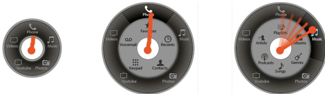
Figure 4: Exploration in Wavelet menus: the user can browse all submenus by performing a continuous circular gesture.
