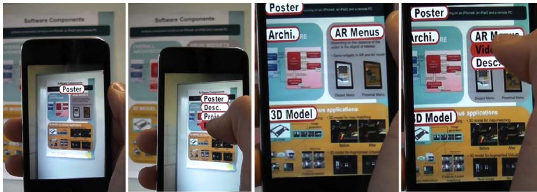
Figure 5.6: Contextual Menus attached to a poster: (Left) From far away, a single global menu is attached to the poster. (Right) From close-up, proximal menus are attached to subparts of the poster and the global menu is available on top of the screen.
