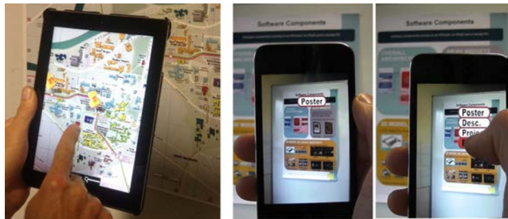
Figure 3.1: Handheld AR pointing tasks: (Left) pointing at a physical location on a remote wall map in order to position an annotation; and (Right) pointing at a digital menu attached to a poster.
