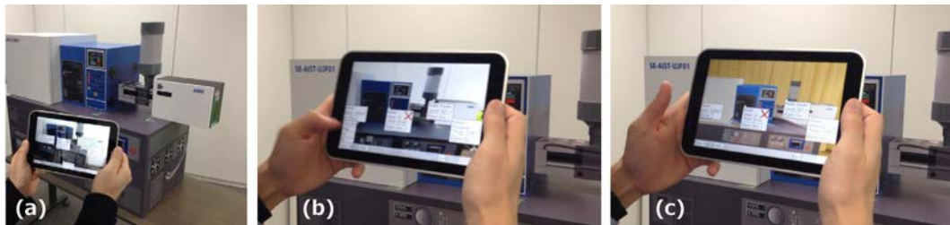
Figure 5.12: Maintenance demonstration. From left to right: (a) Mock-up machine and Windows tablet, (b) AR view of the mock-up machine with augmentations, and (c) Augmented Virtuality mode, showing the 3D model of the machine with augmentations.
