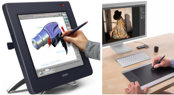
Figure 2. Interactive pen display (direct interaction) vs. Graphics tablet (indirect interaction)
