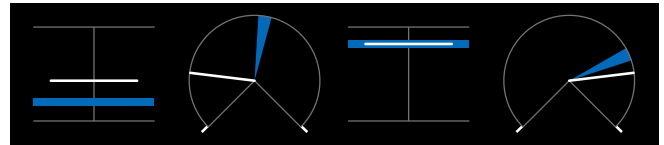
Figure 7. An example of the displays the user saw on the projected screen while carrying out the pursuit task. Widgets on the emergeable are used to control the sliders (far left and centre right) or dials (far right and centre left). There are four positions that controls could be displayed, as illustrated in the image. Each position can display a slider or a dial. Only one (single widget task) or two (dual widget task) widgets were visible at any one time. The widgets on each prototype were rendered in the same positions relative to the large screen. Solid white lines are the user's controller in each case; blue shaded areas are their target.
