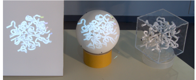
Figure 1. The three methods used to provide visual stimuli in the experiment: on a planar screen (left), on the spherical HPCD (center), and using a physical object (right). All three provided head-coupled stereo.
