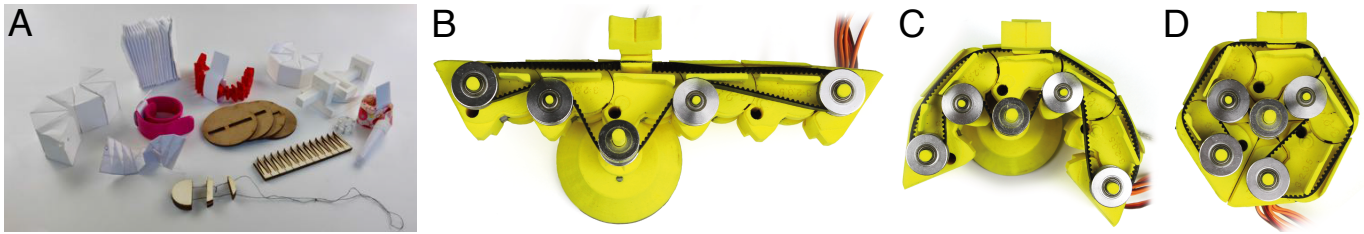
Figure 3. (A) Low-fi prototypes. (B-C-D) KnobSlider working prototype without the top cover to expose the slider's timing belt and the slider mechanism. (B) In slider shape, the movement of timing belt is conveyed through the gears, (C) during transformation, the edges of blocks start to lock the bottom central gear, (D) the edges completely lock the bottom central gear, the rotation of the knob does not affect the timing belt.
