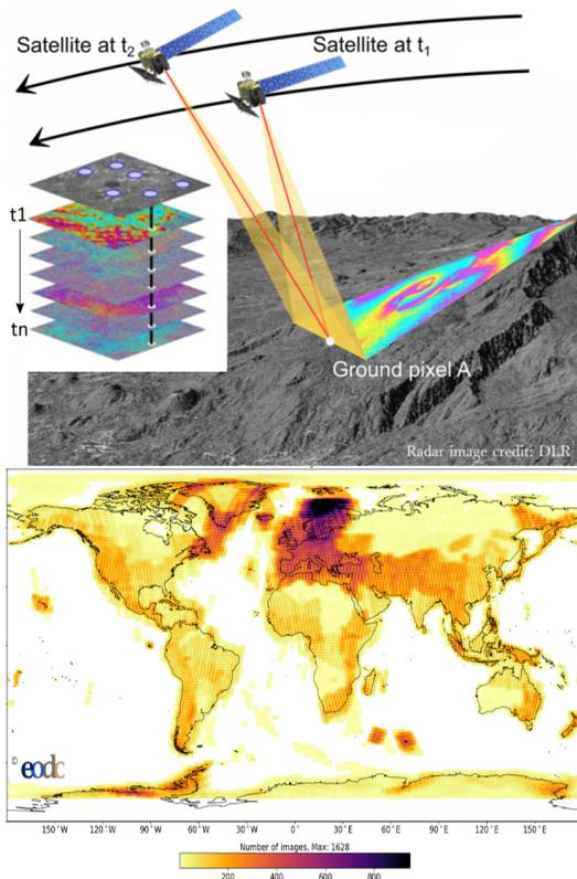
Fig. 1. InSAR Presentation: **top**: the satellites imaging the same place at different times, hence allowing to build a stack of radar interferograms which are differentiation of the phase of radar images. **bottom**. Density of image acquisition. Revisiting time goes up to 2 days in Europe.
